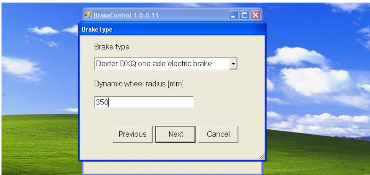
**Enter the Dynamic Wheel Radius, in millimetres, please note this is different for each tire and each brand / type.**
