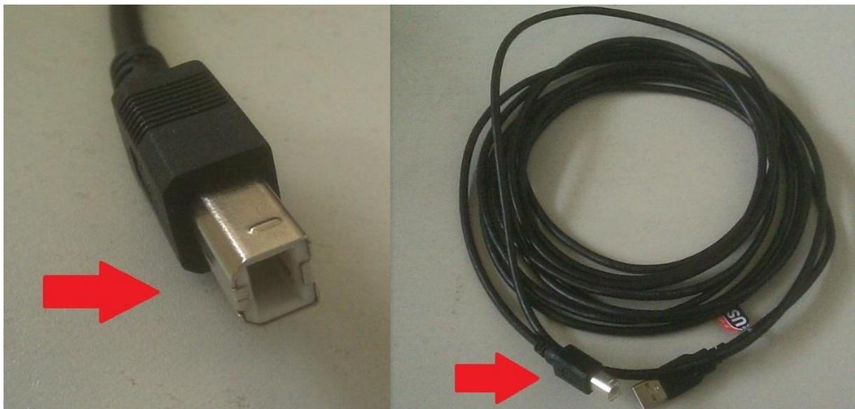
**Unscrew the plug from the brake controller and connect the brake controller to the computer with the USB cable.**
